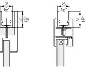
The suspension profile (12915) allows for the use of commercial
